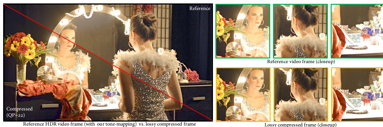
Figure 1: We compare a reference HDR video frame and a lossy compressed frame using our surround-aware CSF model. We compress the original video by three orders of magnitude without perceivable artifacts.
