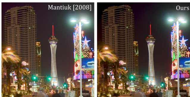
Figure 11: Tone mapped images using Mantiuk's [MDK08] original tone mapping operator (left), and plugging our CSF model (right). For scenes with dark surround luminances, our CSF presents a low sensitivity, therefore it compresses contrast better leading to cleaner images with less residual haze (better seen in the digital version).
