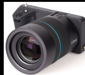
Depth-from-defocus Lytro Illum: Light-field camera
