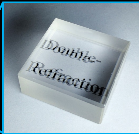
(b) Double refraction in calcite
