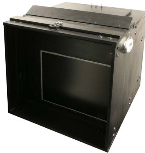
Figure 4.1: A custom-built high-luminance display. The display can produce a luminance of 2\,200\text{ cd/m}^2 when used as an LCD display and up to 30\,000\text{ cd/m}^2 when used with transparencies.
