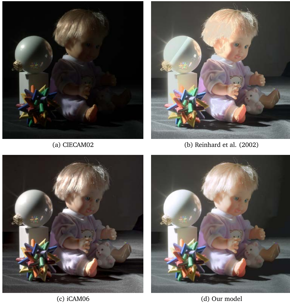
Figure 6.6: Qualitative comparison of visual predictions. Absolute HDR radiance maps are tone-mapped using (a) CIECAM02, (b) Reinhard et al.'s tone-mapping algorithm, (c) the iCAM06 image appearance model, and (d) our colour appearance model. Different from other methods, our model does not struggle with local adaptation artefacts like halos. Estimated peak luminance: 1\,199\text{ cd/m}^2 . Image courtesy of Yuanzhen Li.
