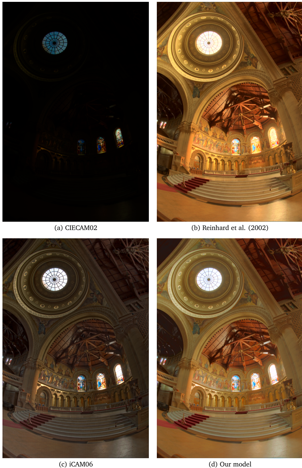
Figure 6.5: Qualitative comparison of visual predictions of (a) CIECAM02, (b) Reinhard et al.'s tone-mapping algorithm, (c) the iCAM06 image appearance model, and (d) our colour appearance model. The target display is assumed to be sRGB with a peak luminance level of 250 \text{ cd/m}^2 and a gamma of 2.2 (dim viewing conditions, adapting luminance is assumed to be 10% of peak luminance). Our model takes into account not only tone but also original colourfulness. Estimated peak luminance: 13\,405 \text{ cd/m}^2 . Image courtesy of Paul Debevec.
